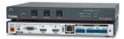
The Extron DTP T USW 233 switcher provides signal extension for up to three sources, sending HDMI or analog video, audio, and control up to 230 feet (70 meters) over a shielded CATx cable to Extron DTP®-enabled products. The HDCP-compliant switcher includes several integrator-friendly features in a low profile enclosure that enables discreet installation in a wide variety of applications.
